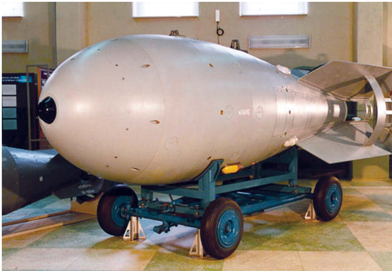
FIGURE 1. THE SLOIKA , or "layer cake," is the informal name for the Soviet Union's first thermonuclear bomb. Although its casing was roughly similar in shape and size to Fat Man, the US atomic bomb dropped on Nagasaki, Japan, in World War II, the Soviet bomb was 20 times as powerful: It detonated with the explosive equivalent of 400 kilotons of TNT. (Courtesy of the Russian Federal Nuclear Center, VNIIEF.)
